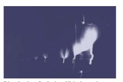
Triggering time of a simple rod lightning conductor
