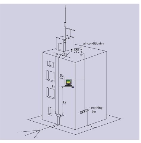
**Example:** a lightning conductor with a down conductor protects a 20-meter high building with protection level I.
